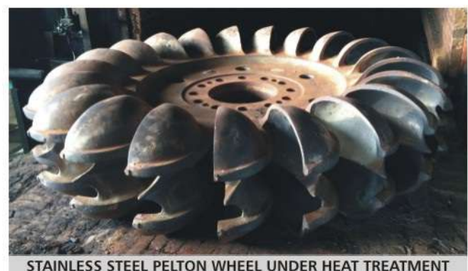
STAINLESS STEEL PELTON WHEEL UNDER HEAT TREATMENT
